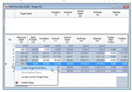
You may now edit any of the exposed cells in the worksheet to adjust the proposal. For example, change the two exposed dogleg rates to **10°/30m** to reduce the sale inclination to **76.622°.**
