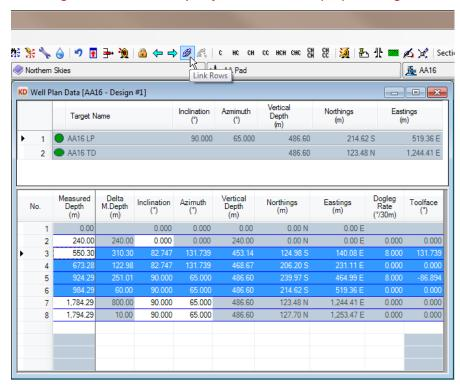
Click on the **Link Rows** button and the lines will be joined to create a **CHCH** stage.
