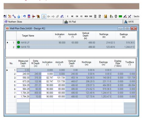
Note that the data is divided into individual lines separated by a blue line and the targets are not attached to any of the individual lines in the proposal data. In this state, you are only able to edit the measured depth, inclination and/or azimuth values.
